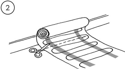
2. The probe wire must NOT cross over the heating element.
