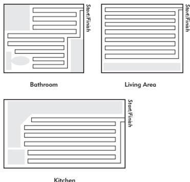
Try and leave the longest wall to last. That way if you have a little too much or too little cable left you can make an easy adjustment by coming a bit further away or going right up close to the wall. Neither option will affect the heating of the room in any way.
