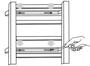
6. Place back brackets covers over back bracket and screw tight from underneath.
