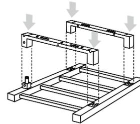
3. Select the 4 M50 x 50mm screws. Place the frame face first on a non scratch surface with the back brackets facing upward. Position the screws through the leg holes tighten to the frame.
