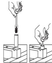
4. Place the Towel Rail on the wall in the desired position and mark your drill hole positions. (Note the rail can move horizontally making it 'Easy to find and fix' to the studs and or drilling between tiles grout lines)
